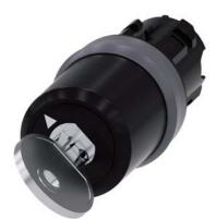
Key-operated switch BKS, 22 mm, round, plastic with metal front ring, lock number S1, with 2 keys, 2 switch positions O-I, latching, actuating angle 90°, 10:30h/13:30h, key removal O+I, with laser labeling, lower case
