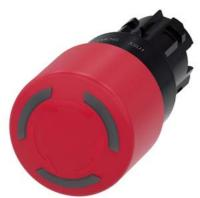
EMERGENCY STOP mushroom pushbutton, illuminable, 22 mm, round, plastic, red, 30 mm, positive latching, acc. to EN ISO 13850, rotate-to-unlatch, with laser labeling, upper case and lower case, always upper case at beginning of line
