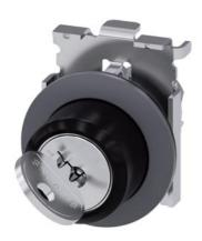
RONIS key-operated switch, 30 mm, round, Metal, matte, front ring for flush installation, lock number SB30, with 2 keys, 2 switch positions O-I, latching, actuating angle  $90^\circ,\,10:30h/13:30h,$  key removal I, possible special locks: SB31, 421, 455, Z=50-unit packaging
