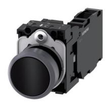
Pushbutton, 22 mm, round, plastic with metal front ring, black, pushbutton, flat, momentary contact type, with holder, 1 NO+1 NC, screw terminal, with laser labeling, upper case
