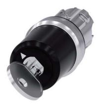
key-operated switch Siemens, 22 mm, round, metal, shiny, lock number SSG10, with 2 keys, 2 switch positions O<I, momentary contact type, actuating angle 45°, 10:30h/12h, key removal O, with laser labeling, inscription or symbol customer-specific selection with SIRIUS ACT configurator (CIN)
