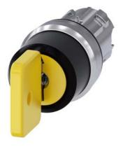
Key-operated switch O.M.R, 22 mm, round, metal, shiny, lock number 73033, yellow, with 2 keys, 3 switch positions I>O<II, momentary contact on the left, latching on the right, actuating angle 2x45°, 10:30h/12h/13:30h, Key removal II, with laser labeling, inscription or symbol Customer-specific selection with SIRIUS ACT configurator (CIN)
