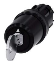
Key-operated switch , 22 mm, round, plastic, special lock, with 2 keys, 3 switch positions I-O<II, left latching, right momentary contact type, actuating angle 2x45°, 10:30h/12h/13:30h, Key removal I
