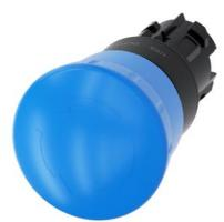
Mushroom pushbutton, 22 mm, round, plastic, blue, 40 mm, positive latching, acc. to EN ISO 13850, rotate-to-unlatch, with laser labeling, symbol number according to ISO 7000 or IEC 60417
