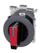
Selector switch, illuminable, 30 mm, round, Metal, matte, red, selector switch, short, front ring for flush installation, 3 switch positions I-O-II, latching, actuating angle 2x45°, 10:30h/12h/13:30h, with laser labeling, inscription or symbol Customer-specific selection with SIRIUS ACT configurator (CIN)
