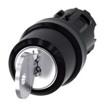
RONIS key-operated switch, 22 mm, round, plastic, lock number SB30, with 2 keys, 3 switch positions I-O-II, latching, actuating angle 2x45°, 10:30h/12h/13:30h, key removal O, possible special locks: SB31, 421, 455 Z=50-unit packaging
