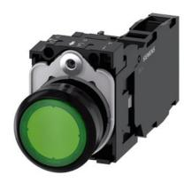
Illuminated pushbutton, 22 mm, round, plastic, green, pushbutton, flat, momentary contact type, with holder, 1 NO+1 NC, LED module with integrated LED 110 V AC, screw terminal, Z=20-unit packaging
