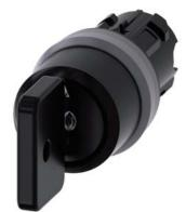
Key-operated switch O.M.R, 22 mm, round, plastic with metal front ring, lock number 73034, black, with 2 keys, 3 switch positions I-O-II, latching, actuating angle 2x45°, 10:30h/12h/13:30h, Key removal I+O+II, with laser labeling, lower case
