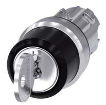
RONIS key-operated switch, 22 mm, round, metal, shiny, lock number SB30, with 2 keys, 3 switch positions I-O-II, latching, actuating angle 2x45°, 10:30h/12h/13:30h, key removal O+I, possible special locks: SB31, 421, 455, with laser labeling, upper case and lower case, always upper case at beginning of line
