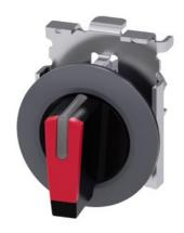
Selector switch, illuminable, 30 mm, round, Metal, matte, red, selector switch, short, front ring for flush installation, 3 switch positions I>O<II, momentary contact type, actuating angle 2x45°, 10:30h/12h/13:30h, with laser labeling, lower case
