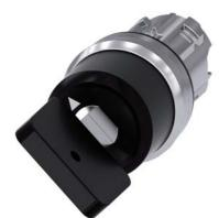
key-operated switch Siemens, 22 mm, round, metal, shiny, lock no. VL5, with 2 keys, 2 switch positions O<I, momentary contact type, actuating angle 45°, 10:30h/12h, key removal O, with laser labeling, lower case
