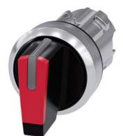
Selector switch, illuminable, 22 mm, round, metal, shiny, red, selector switch, short, 3 switch positions I-O<II, left latching, right momentary contact type, actuating angle 2x45°, 10:30h/12h/13:30h, Z=50-unit packaging
