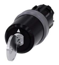
Key-operated switch BKS, 22 mm, round, plastic with metal front ring, lock number S1, with 2 keys, 3 switch positions I-O<II, left latching, right momentary contact type, actuating angle  $2x45^{\circ}$ , 10:30h/12h/13:30h, key removal O+I, with laser labeling, upper case and lower case,
