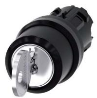
RONIS key-operated switch, 22 mm, round, plastic, lock number SB30, with 2 keys, 3 switch positions I-O<II, left latching, right momentary contact type, actuating angle 2x45°, 10:30h/12h/13:30h, key removal I, possible special locks: SB31, 421, 455 Z=50-unit packaging
