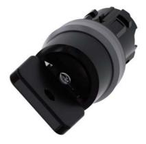
Key-operated switch O.M.R, 22 mm, round, plastic with metal front ring, lock number 73034, black, with 2 keys, 2 switch positions O-I, latching, actuating angle 90°, 10:30h/13:30h, key removal O+I, with laser labeling, upper case
