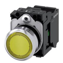
Illuminated pushbutton, 22 mm, round, metal, shiny, yellow, pushbutton, flat, momentary contact type, with holder, 1NO, LED module with integrated LED 24 V AC/DC, spring-type terminal, with laser labeling, symbol number according to, ISO 7000 or IEC 60417
