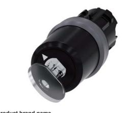
Key-operated switch BKS, 22 mm, round, plastic with metal front ring, lock number S1, with 2 keys, 2 switch positions O-I, latching, actuating angle 90°, 10:30h/13:30h, key removal O+I, with laser labeling, upper case and lower case, always upper case at the beginning of the word
