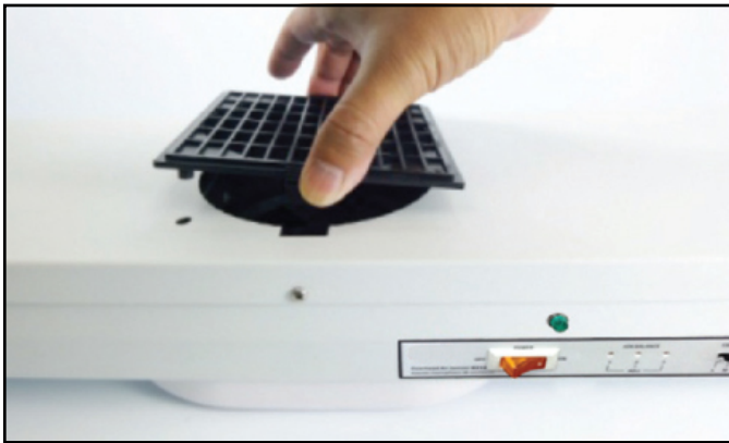
Figure 7. Remove the back grill by removing the screws, pressing the latch tabs on each side and pulling off.
