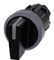
Illuminable selector switch, 22 mm, round, plastic with metal front ring, black, Selector switch short, 3 switch positions I-O<II, left latching, momentary contact type on the right, actuating angle 2x45°, 10:30 /12 /13:30, Z=50-unit packaging
