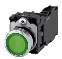
Illuminated pushbutton, 22 mm, round, Metal, shiny, green, pushbutton, flat, momentary contact type, with holder, 1 NO+1 NC, LED module with integrated LED 230 V AC, screw terminal, with laser labeling, inscription or symbol Customer-specific selection with SIRIUS ACT configurator (CIN)
