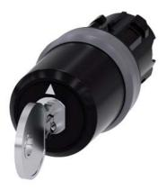
key-operated switch Siemens, 22 mm, round, plastic with metal front ring, lock number SSG10, with 2 keys, 3 switch positions I>O<II, momentary contact type, actuating angle  $2x45^{\circ}$ , 10:30h/12h/13:30h, key removal O, with laser labeling, upper case and lower case, always upper case at the beginning of the word
