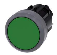
Pushbutton, 22 mm, round, plastic with metal front ring, green, pushbutton, flat, latching, Push-to-release mechanism, with laser labeling, upper case
