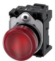
Indicator lights, 22 mm, round, metal, shiny, red, lens, smooth, with holder, LED module with integrated LED 24 V AC/DC, spring-type terminal, Z=20-unit packaging
