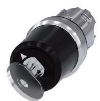
Key-operated switch BKS, 22 mm, round, metal, shiny, lock number S1, with 2 keys, 2 switch positions O-I, latching, actuating angle 90°, 10:30h/13:30h, key removal O+I, with laser labeling, lower case
