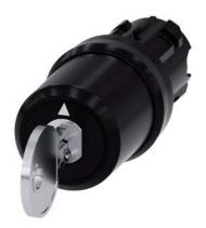
key-operated switch Siemens, 22 mm, round, plastic, special lock, with 2 keys, 3 switch positions I>O<II, momentary contact type, actuating angle 2x45°, 10:30h/12h/13:30h, key removal O
