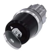
Key-operated switch BKS, 22 mm, round, metal, shiny, lock number S1, with 2 keys, 2 switch positions O-I, latching, actuating angle  $90^\circ$ , 10:30h/13:30h, key removal I, with laser labeling, inscription or symbol Customer-specific selection with SIRIUS ACT configurator (CIN)
