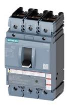
circuit breaker 3VA5 UL frame 250 breaking capacity class H 65kA @ 480 V 3-pole, line protection TM230, FTAM, In=100A overload protection Ir=100A fixed short-circuit protection Ii=5...10 x In UL489 SB (naval), 50 deg. cel. cable connection on both sides
