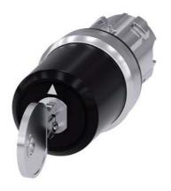
Key-operated switch BKS, 22 mm, round, metal, shiny, lock number S1, with 2 keys, 3 switch positions I>O<II, momentary contact type, actuating angle  $2x45^{\circ}$ , 10:30h/12h/13:30h, key removal O, with laser labeling, upper case and lower case, always upper case at beginning of line
