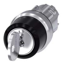
RONIS key-operated switch, 22 mm, round, metal, shiny, lock number SB30, with 2 keys, 3 switch positions I-O<II, left latching, right momentary contact type, actuating angle 2x45°, 10:30h/12h/13:30h, key removal I, possible special locks: SB31, 421, 455, with laser labeling, upper case and lower case, always upper case at the beginning of the word
