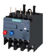
Overload relay 3.5...5.0 A Thermal For motor protection Size S00, Class 10 Contactor mounting Main circuit: Ring cable lug Auxiliary circuit: ring cable lug Manual-Automatic-Reset
