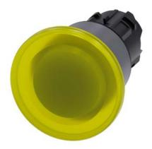
Illuminated mushroom pushbutton, 22 mm, round, plastic with metal front ring, yellow, 40 mm, latching, pull-to-unlatch mechanism, with laser labeling, symbol number according to, ISO 7000 or IEC 60417
