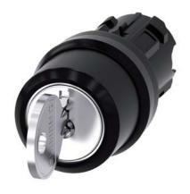
RONIS key-operated switch, 22 mm, round, plastic, lock number SB30, with 2 keys, 3 switch positions I-O<II, left latching, right momentary contact type, actuating angle 2x45°, 10:30h/12h/13:30h, key removal I, possible special locks: SB31, 421, 455, with laser labeling, upper case and lower case, always upper case at beginning of line
