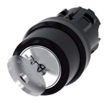
RONIS key-operated switch, 22 mm, round, plastic, lock number SB30, with 2 keys, 2 switch positions O<I, momentary contact type, Actuating angle 45°, 10:30h/12h, key removal O, possible special locks: SB31, 421, 455, with laser labeling, upper case and lower case, always upper case at beginning of line
