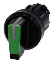
Selector switch, illuminable, 22 mm, round, plastic, green, selector switch, short, 3 switch positions I>O<II, momentary contact type, actuating angle 2x45°, 10:30h/12h/13:30h, with laser labeling, upper case and lower case, always upper case at beginning of line
