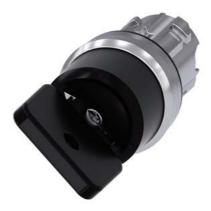
Key-operated switch O.M.R, 22 mm, round, metal, shiny, lock number 73034, black, with 2 keys, 2 switch positions O<I, momentary contact type, Actuating angle 45°, 10:30h/12h, key removal O, with laser labeling, upper case
