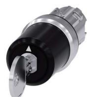
Key-operated switch BKS, 22 mm, round, metal, shiny, lock number S1, with 2 keys, 3 switch positions I-O-II, latching, actuating angle 2x45°, 10:30h/12h/13:30h, Key removal I+O+II, with laser labeling, lower case
