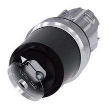
Key-operated switch IKON, 22 mm, round, metal, shiny, lock number 360012K1, with 2 keys, 2 switch positions O-I, latching, actuating angle 90°, 10:30h/13:30h, key removal O+I, with laser labeling, upper case and lower case, always upper case at beginning of line
