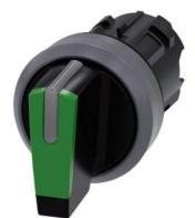
Selector switch, illuminable, 22 mm, round, plastic with metal front ring, green, selector switch, short, 3 switch positions I>O<II, momentary contact on the left, latching on the right, actuating angle  $2x45^{\circ}$ , 10:30h/12h/13:30h, Z=50-unit packaging
