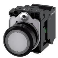
Illuminated pushbutton, 22 mm, round, plastic, clear, pushbutton, flat, momentary contact type, with holder, 1NO, LED module with integrated LED 110 V AC, spring-type terminal, with laser labeling, upper case
