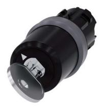
Key-operated switch BKS, 22 mm, round, plastic with metal front ring, lock number S1, with 2 keys, 2 switch positions O-I, latching, actuating angle 90°, 10:30h/13:30h, key removal I, Z=50-unit packaging
