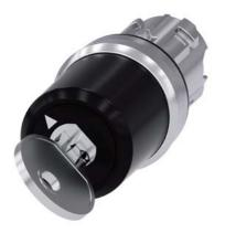
key-operated switch Siemens, 22 mm, round, metal, shiny, lock no. LSG1, with 2 keys, 2 switch positions O<I, momentary contact type, actuating angle 45°, 10:30h/12h, key removal O, with laser labeling, lower case
