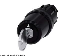
key-operated switch Siemens, 22 mm, round, plastic, lock number SSG10, with 2 keys, 3 switch positions I>O<II, momentary contact type, actuating angle  $2x45^{\circ}$ , 10:30h/12h/13:30h, key removal O, with laser labeling, upper case and lower case, always upper case at the beginning of the word
