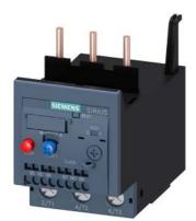
Overload relay 47...57 A Thermal For motor protection Size S2, Class 10 Contactor mounting Main circuit: Screw Auxiliary circuit: spring-type terminal Manual-Automatic-Reset
