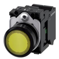
Illuminated pushbutton, 22 mm, round, plastic, yellow, pushbutton, flat, momentary contact type, with holder, 1NO, LED module with integrated LED 24 V AC/DC, spring-type terminal, with laser labeling, symbol number according to, ISO 7000 or IEC 60417
