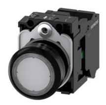
Illuminated pushbutton, 22 mm, round, plastic, clear, pushbutton, flat, momentary contact type, with holder, 1NO, LED module with integrated LED 230 V AC, spring-type terminal, with laser labeling, lower case
