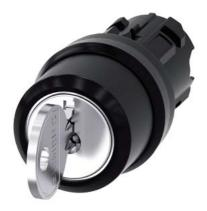
RONIS key-operated switch, 22 mm, round, plastic, lock number SB30, with 2 keys, 3 switch positions I-O-II, latching, actuating angle 2x45°, 10:30h/12h/13:30h, key removal O+I, possible special locks: SB31, 421, 455, with laser labeling, upper case and lower case, always upper case at beginning of line
